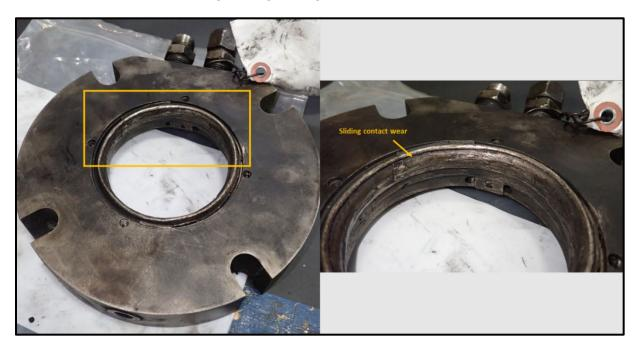
**Figure 24.** Smeared metal on inside surface of seal gland that indicates sliding contact with the pump shaft. (Credit: Stress Engineering)
