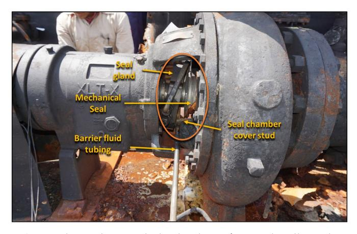
**Figure 26.** Tank 80-8 circulation pump. This photo shows the point of separation observed between the mechanical seal gland and seal chamber cover where the butane-enriched naphtha product released. (Credit: CSB).
