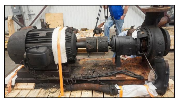
**Figure 22.** Tank 80-8 pump removed from ITC Deer Park terminal. Pictured is the pump kit on a pallet, as removed from the incident site. (Credit: CSB)
