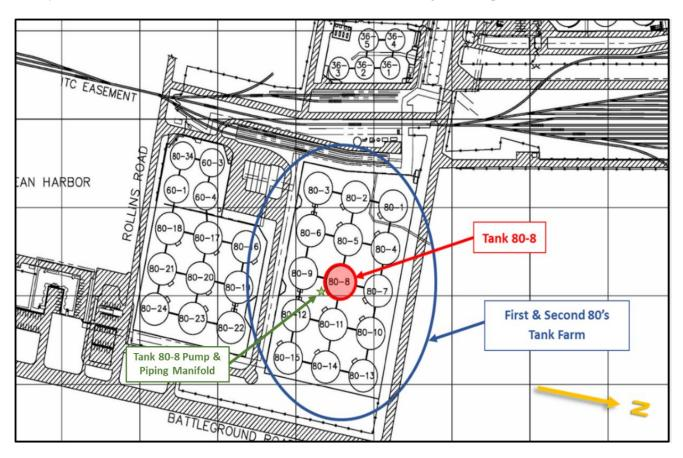
**Figure 5.** Plot plan of 80's truck rack. Excerpt from overall plot plan for the ITC Deer Park terminal showing the location of the 80's truck rack and First & Second 80's tank farm. (Credit: ITC, annotations by CSB).
