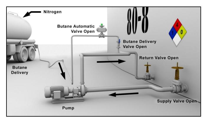
**Figure 6.** Simplified schematic showing ITC's butane injection system prior to 2016. The arrows in the figure show the butane flow direction and the naphtha product circulation path through the piping. Note: schematic not to scale. (Credit: CSB)
