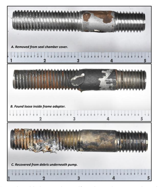
**Figure 27.** Three seal chamber cover studs recovered from Tank 80-8 circulation pump, post-cleaning. The longer threaded ends passed through the slots in the seal gland, while the shorter threaded ends were engaged in the seal chamber cover. (Credit: Stress Engineering)
