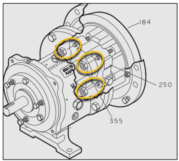
**Figure 25.** Cutaway drawing of *Goulds* chemical process pump showing the locations of three of the four gland nuts that held the seal gland in place against the seal chamber cover. *Note: fourth gland nut is not visible in drawing.* [Credit: *Goulds,* annotations by CSB]
