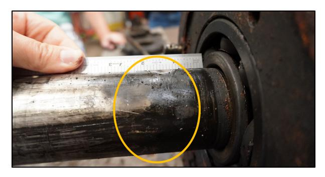
**Figure 23.** The severe abrasive wear damage observed on the Tank 80-8 pump shaft adjacent to inboard side of bearing housing, on August 30, 2019. (Credit: CSB)
