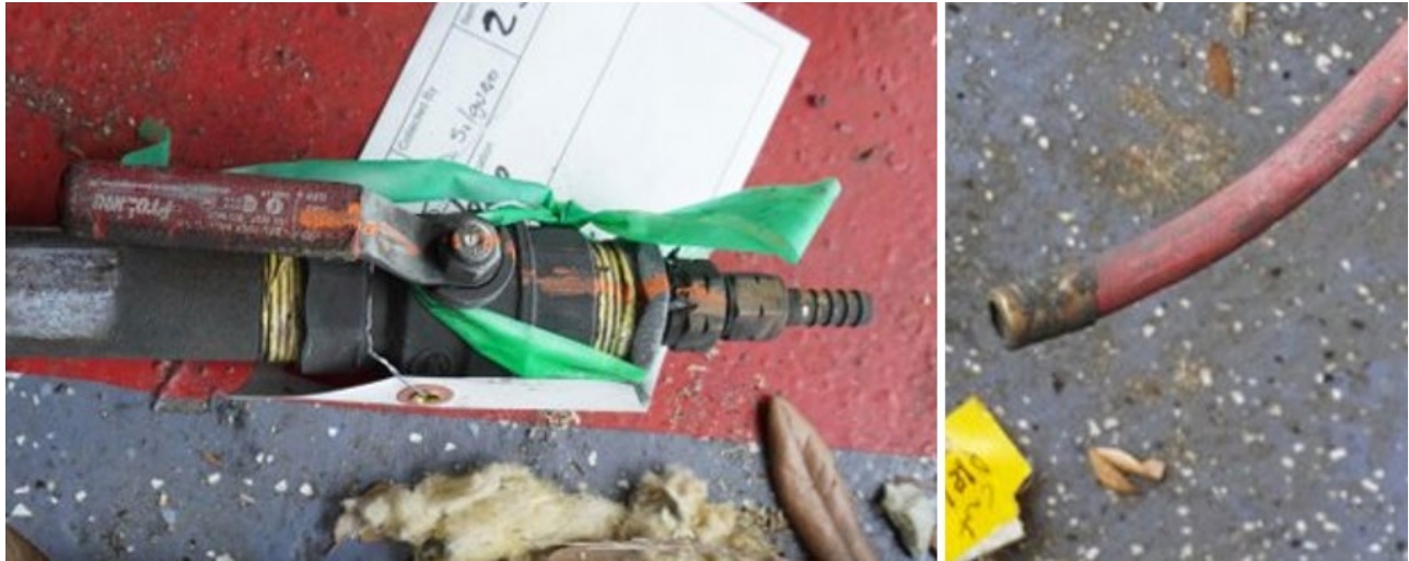
Figure 20. Disconnected Welding Hose from Booth 4. (Source: CSB)
